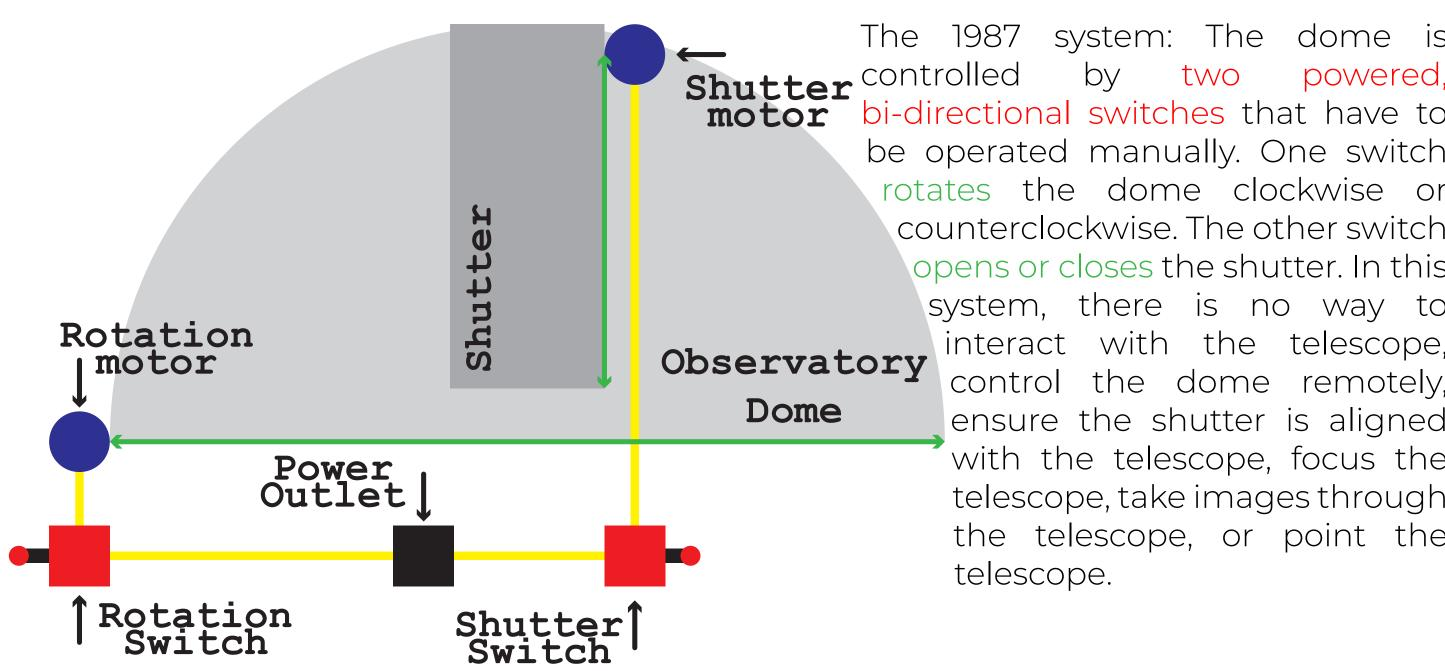
**Project** Goal: Rebuild observatory Primary control system from the ground up, allowing for full remote functionality.
