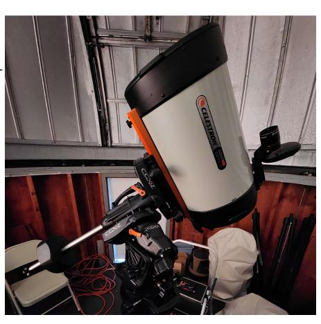
**Smart Telescope Mount:** Accurately and precisely controlling the telescope is integral for capturing good astronomical data. Our Celestron CGX-L Smart Telescope Mount is an amazing piece of equipment that, through the help of guiding, is able to accurately track objects through the sky within 0.5 arcseconds of error (that's 1/7,200th of a single degree of accuracy!)
